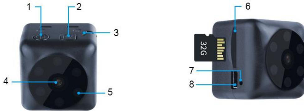
1.Power button; 2.M-Mode button; 3.Indicator light ; 4.Lens; 5.IR(Infrared night vision lights); 6.TF Card; 7.Reset button; 8.USB
