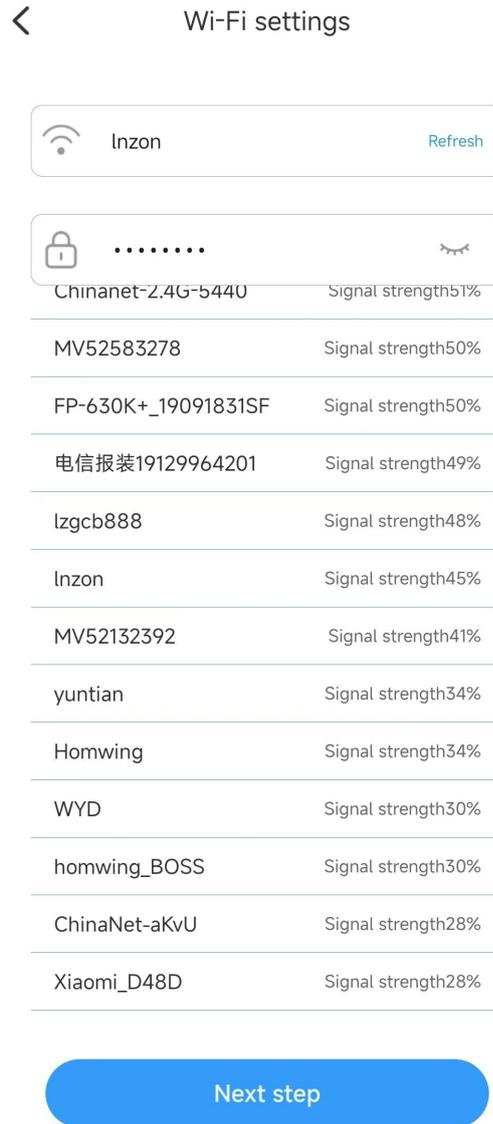
Two minutes later, the device will connect to the network. If an incorrect password is entered during the operation, the device will restart normally but will not successfully connect to the network. You can reset the device to factory settings and return to local mode by long pressing the "R" button for 5 seconds and then releasing it. Perform the operation again from step "1".
